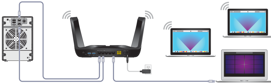
Figure 7. Ethernet port aggregation
